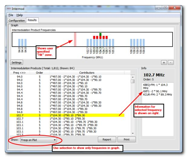
The frequencies shown in blue indicate products of greater than third order. The ones displayed in red indicate second and third order products. The frequencies shown in green indicate a fundamental frequency of one of the transmitters included in the study.
