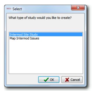
**Intermod Site Study** – Use this to determine the intermodulation products for a set of transmitters that are in the same location.
